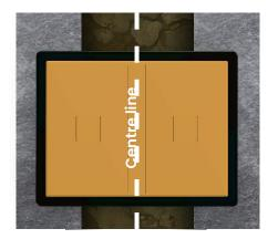
Always position the trench cover board **centrally** over the trench as illustrated.
