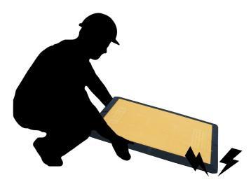
When fitting the product in place, never drop the product, gently lower it in place. Never lift or move with machinery. Never walk the product leading edge.
